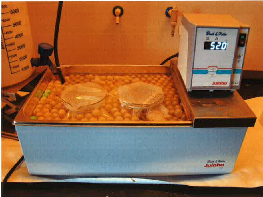
Figure 1: The test bath with the two panels immersed in the water/fuel mixture in the glasses.
